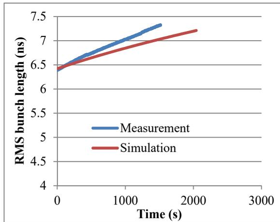
Figure 1: Comparison between measured and simulated bunch length evolution over ~30 minutes.
