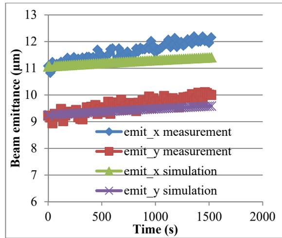
Figure 3: Transverse emittances measured by IPMs at injection and simulated transverse emittance evolution for coupled case with 9 MHz cavity.
