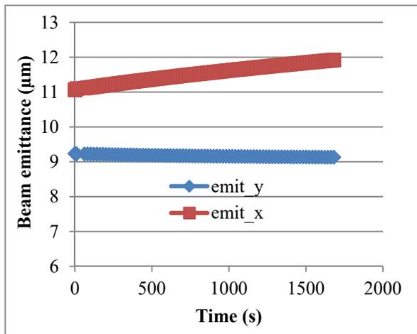
Figure 2: Transverse emittance evolution simulated by BETACOOOL for the decoupled case with 9 MHz RF system; the horizontal emittance is in red and vertical emittance in blue.
