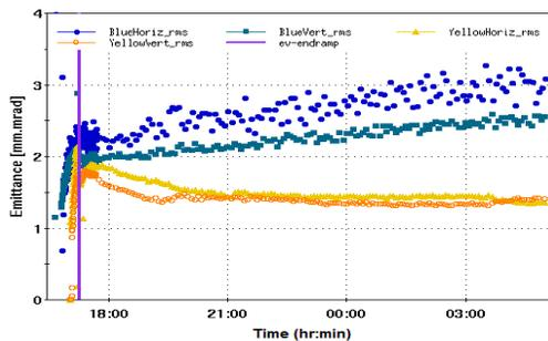
Figure 1: Beam transverse emittance evolution of the two beams for the 39 GeV/n program. The gold beam emittances in both planes (the yellow and orange) were reduced with only vertical cooling engaged.
