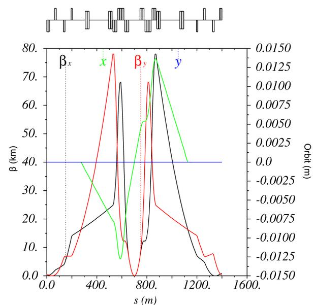
Figure 2: Twiss Functions and Orbit for 0.3 m  $\beta^*$  Round Optics
