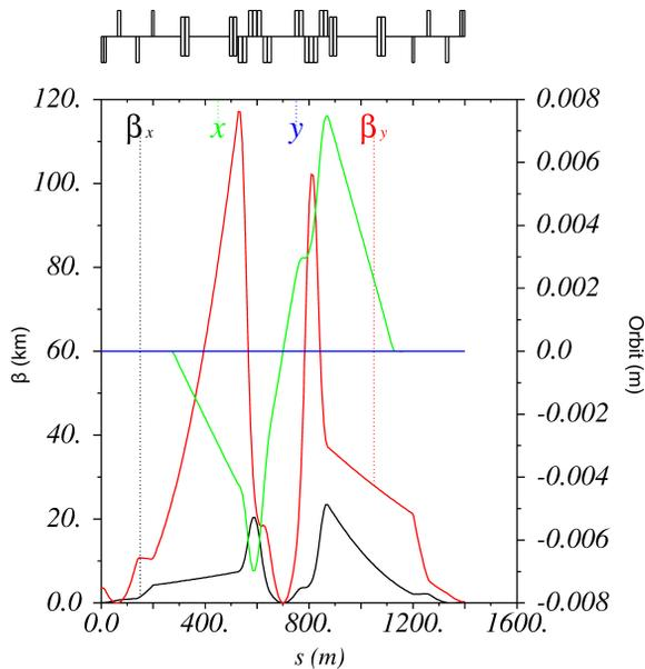
Figure 3: Twiss Functions and Orbit for  $0.2 \times 1$  m  $\beta^*$  Flat Optics
