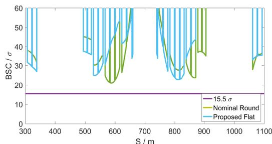
Figure 4: Plot Showing BSC for Ultimate Round and Proposed Flat Optics
