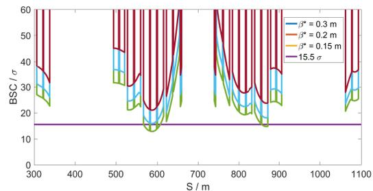
Figure 5: Plot Showing BSC for  $\beta^* = 0.15, 0.2$  and  $0.3$  Round Optics
