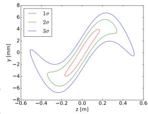
Figure 2:  $1\sigma$ ,  $2\sigma$  and  $3\sigma$  (red, green and blue respectively) of the crabbed beam at the HT monitor (55 GeV, V=6.8 MV).
