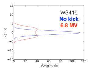
Figure 5: Vertical beam profile without (blue) and with a kick corresponding to 6.8 MV (red).
