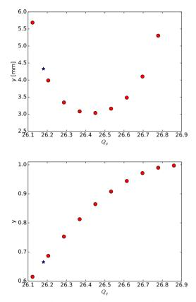
Figure 1: Absolute (top) and normalised (bottom) vertical CO offset at the HT monitor as a function of  $Q_y$ ; blue star: vertical operational tune (26.18).
