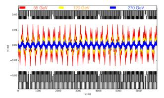
Figure 3:  $3\sigma$  beam of 55, 120 and 270 GeV. For all three cases the beam is within the aperture limits.
