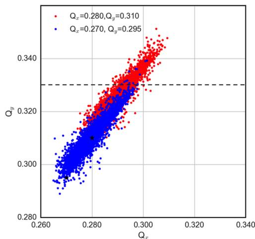
Figure 2: Tune footprints evaluated for a LHC bunch at injection including the effect of octupoles powered at 26 A,  $Q'_{x,y}$  at 15 units, and EC in dipole and quadrupole magnets. The dashed line represents the third order resonance  $Q_y=.33$ .
