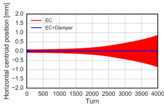
Figure 5: Evolution of the horizontal bunch centroid position with and without the transverse feedback system. The EC density in dipoles has been assumed equal to  $9 \cdot 10^{11} \text{ e-/m}^3$ .
