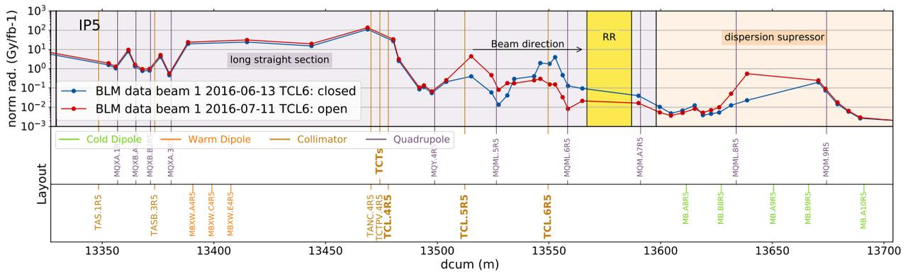
Figure 4: Dose measurements normalized with the integrated luminosity for the right side of the collision point in IR5 (CMS). The changes in the collimator settings lead to significant changes in the radiation levels downstream of the collimators.
