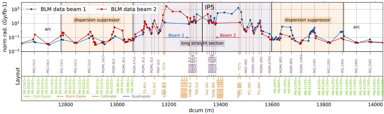
Figure 3: Dose measurements normalized with the integrated luminosity for beam 1 and beam 2 in IR5 of the LHC. Beneath the dose plot the magnet layout with the TCL collimators are shown.
