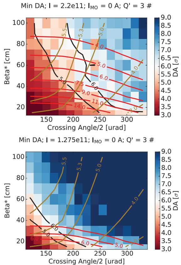
Figure 2: Multi-parametric scans of minimum DA in beam sigma for various values of  $\beta^*$  and half crossing angle for the start (top) and the end (bottom) of the levelling process. The superimposed curves correspond to the various contours of Dynamic Aperture (black), Luminosity (red) and r.m.s. length of the luminous region (gold). The study was performed with 3 units of chromaticity and the octupoles off.
