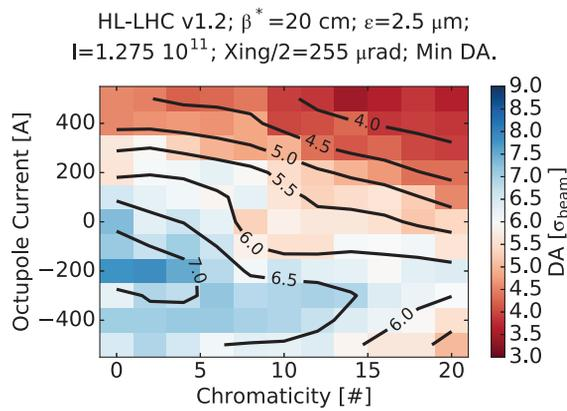
Figure 1: DA response to octupoles and chromaticity for the nominal crossing angle of  $510$   $\mu\text{rad}$  and end-of-levelling settings with head-on collisions in LHCb and  $5\sigma$  separated beams in Alice. The negative setting for octupoles improves the DA, allowing for a larger chromaticity and/or reduced crossing angle.
