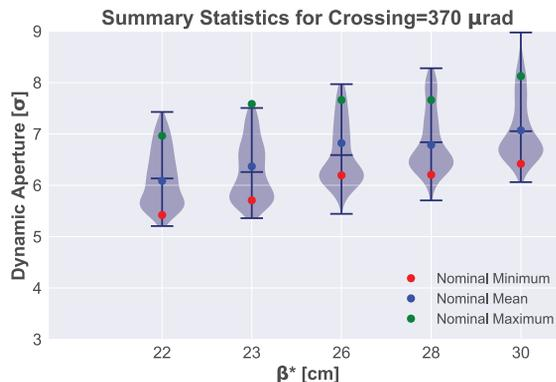
Figure 4: The DA as a function of the  $\beta^*$  is illustrated for 370  $\mu$ rad crossing angle. The three bar points for each violin correspond to the minimum, average and maximum value of the statistical population. The shaded area represents the density of seeds presenting the same DA. The red bullets on top of each violin correspond to the minimum DA of the case without errors.
