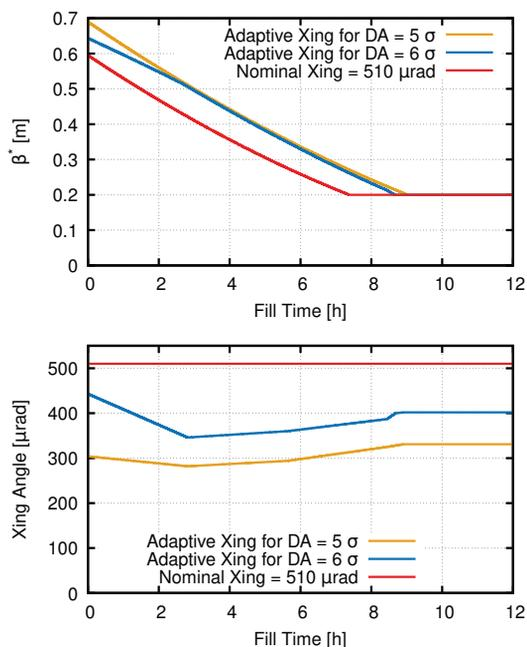
Figure 3: The evolution of  $\beta^*$  (top) and crossing angle (bottom) as a function of time for the relaxed and the aggressive scenarios, with round emittance. The nominal case with the crossing angle fixed at 510  $\mu$ rad is also shown.
