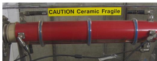
Figure 1: SPEAR3 ceramic beam excitation module.
