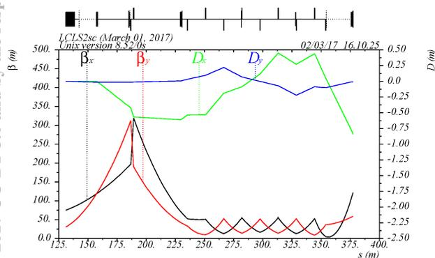
Figure 5: Optics functions in the DASEL beamline.
