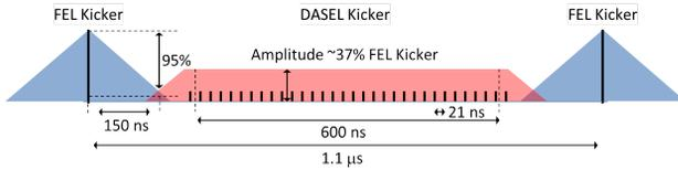
Figure 2: LCLS-II beam structure and kicker pulse. Large bars are FEL bunches, small bars are dark current buckets, blue is FEL kicker pulse, and red is DASEL kicker pulse.
