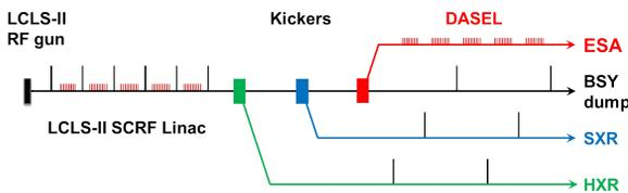
Figure 3: Schematic of the FEL and DASEL kicker system.
