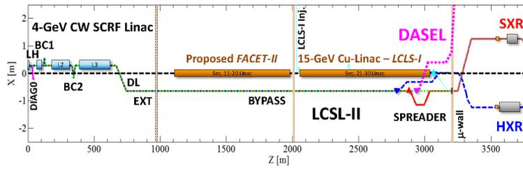
Figure 1: Top view layout of LCLS beamlines, where HXR is dash blue, SXR is solid red, and DASEL is dash pink.
