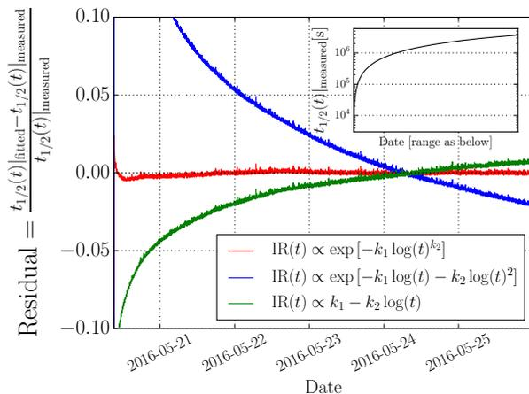
Figure 2: Fit residuals for different models of  $t_{1/2}(t)$  using the measured IR decay on PMIU.202 in LSS2.
