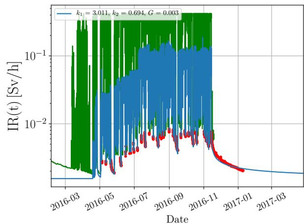
Figure 3: IR model (blue) fitted to measured filtered data (red): first 5 h of data after beam stops and saturated data are filtered from the raw data (green),  $\Delta t = 0.5$  h.
