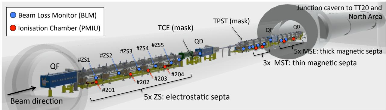
Figure 1: LSS2 slow extraction region towards the TT20 transfer line and the NA [6].
