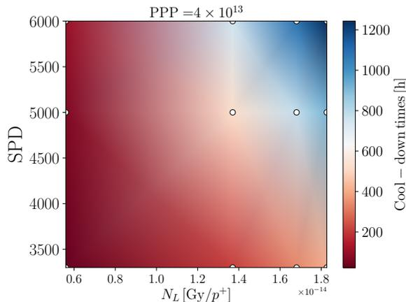
Figure 4: Parametric study of waiting times for the reference intervention: ZS2 tank exchange at 5 mSv collective dose.
