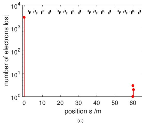
Figure 2: Electron lose under during injection. (a) Simulation in the  $x$ - $x'$  plane; (b) simulation in the  $y$ - $y'$  plane; (a) simulation in the  $x$ - $dp/p$  plane.
