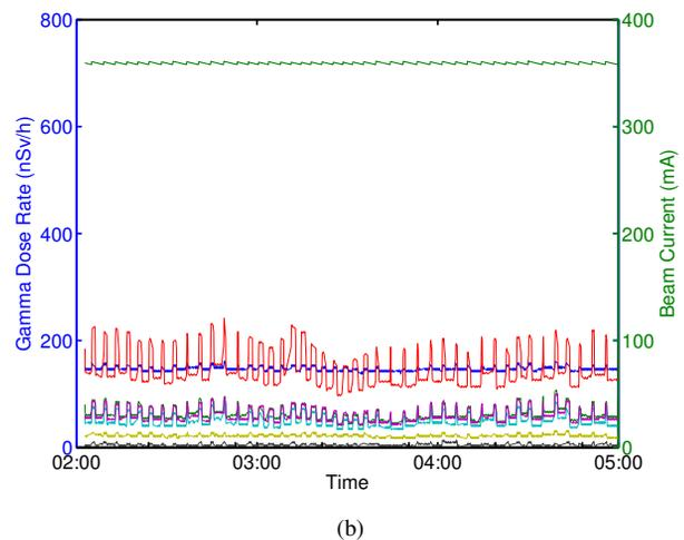
Figure 5: The measured radiation dose rate. (a) Before the additional shielding wall installed; (b) after the additional shielding wall installed
