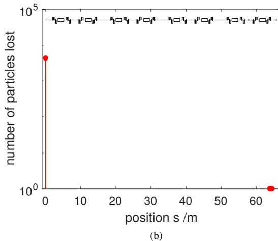
Figure 4: Electron loss with different kicker angles. (a) kicking angle equals 0.1 mrad; (b) kicking angle equals 0.3 mrad.
