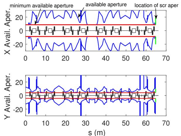
Figure 1: (color) The available aperture along the HLS storage ring. (up) horizontal direction; (down) vertical direction.
