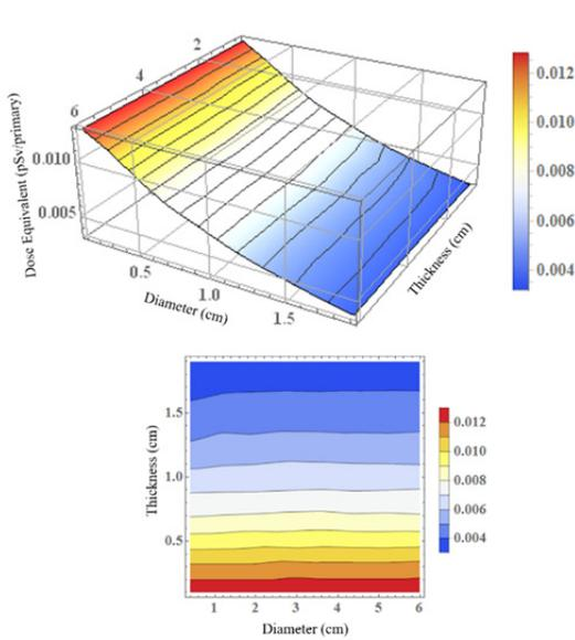
Figure 4: Dose equivalent of generated photon with tantalum target as function of diameter and thickness.
