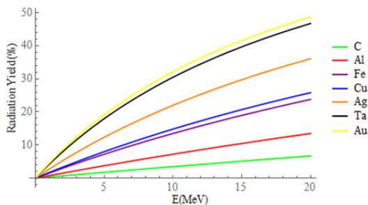
Figure 7: Radiation yield as a function of material atomic number and the kinetic energy of incident electrons.
