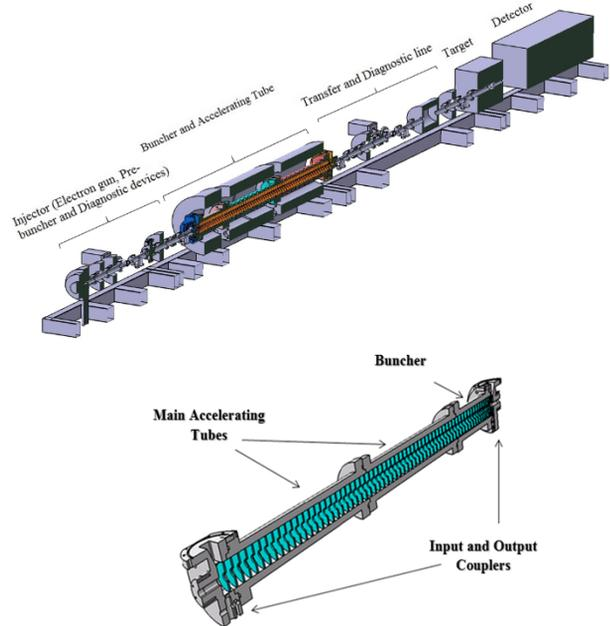
Figure 1: Layout of IPM E-Linac [1].
