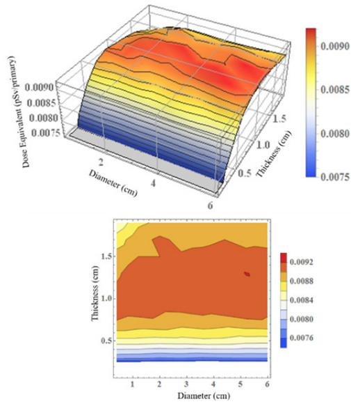
Figure 5: Dose equivalent of generated photon with carbon target as function of diameter and thickness.
