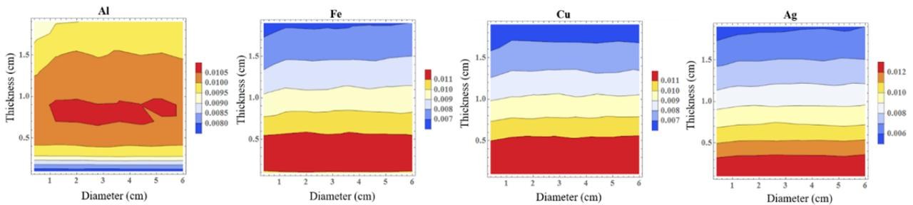
Figure 6: Dose equivalent of generated photon with Al, Fe, Cu and Ag as function of target diameter and thickness.
