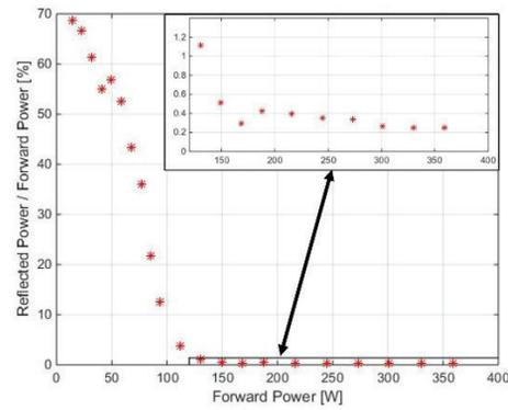
Figure 3: Fraction of reflected microwave power vs injected
