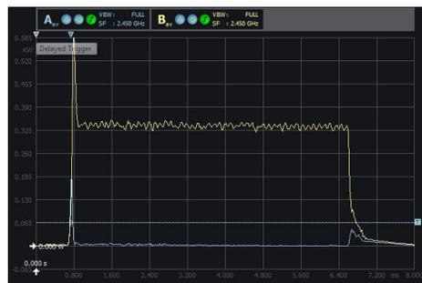
Figure 5: Forward power  $P_{FW}$  (yellow curve) and reflected Power  $P_{Refl}$  (blue curve) when the ATU is in automatic mode and gas flow rate is 1.41 sccm.
