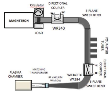
Figure 1: PS-ESS 2.45 GHz microwave injection block scheme.
