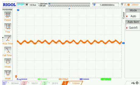
Figure 2: Ripple measurement of  $\pm 0.5\%$  ( $P_{FW}=2$  kW)
