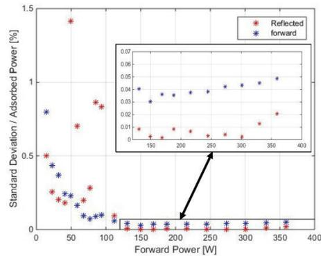
Figure 4: Stability of microwave absorbed power.
