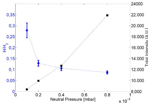
Figure 4: Dependence of the  $n_H/n_{H_2}$  ratio on the pressure.
