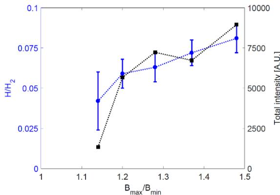
Figure 5: Dependence of the  $n_H/n_{H_2}$  ratio on the  $B_{max}/B_{min}$  ratio.
