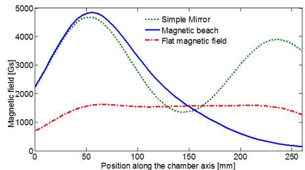
Figure 1: Magnetic field profiles that can be generated by the FPT.
