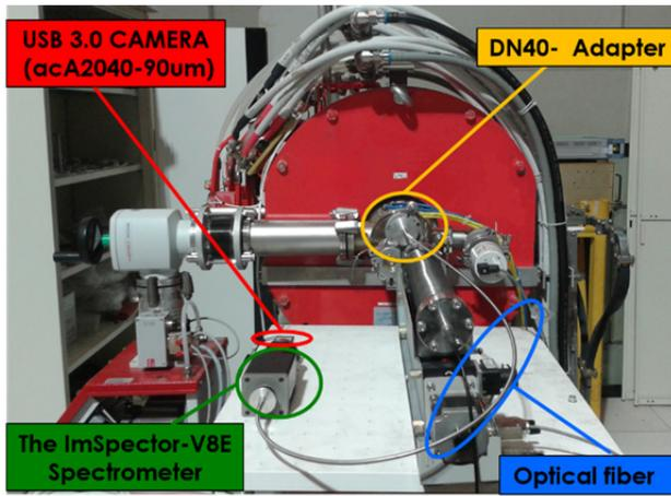
Figure 2: A view of the FPT and the OES set-up.
