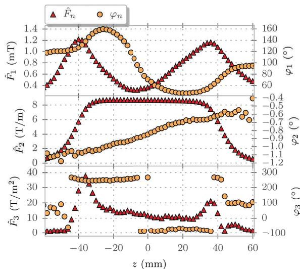
Figure 1: Results of the circular magnetic field measurements of QG1. Shown are the first three multipole strengths  $\hat{F}_{n=1,2,3}$  and the according phases  $\varphi_{n=1,2,3}$  along the nominal beam axis. The yokes reach from  $\pm 40$  mm.
