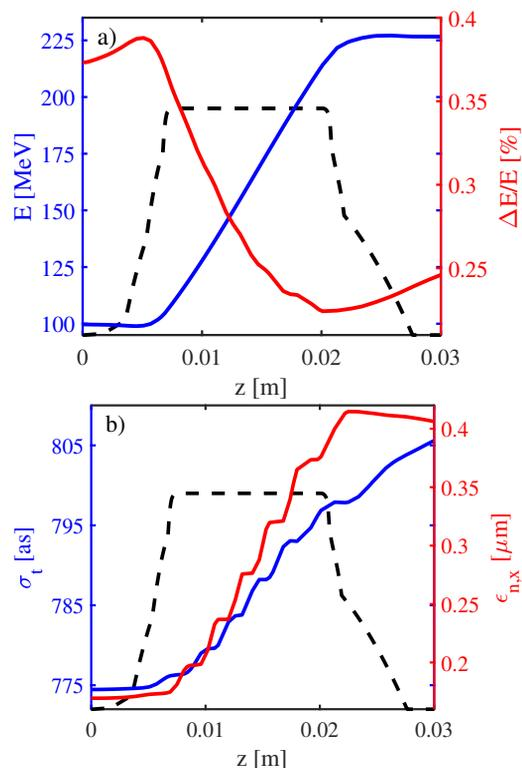
Figure 3: Evolution of the electron beam properties during acceleration in an external injection LWFA plasma setup based on a 2D OSIRIS simulation. The black, dashed line represents the shape of the plasma density profile.
