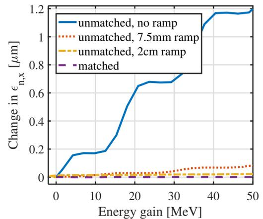
Figure 2: Emittance evolution during acceleration of matched and unmatched beams with plasma profiles with varying density upramp lengths.
