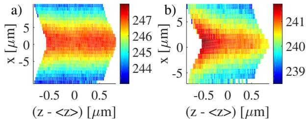
Figure 1: Energy distribution (in MeV) across the witness beam in  $z$  and  $x$  for a beamloading optimised case (a) and a non-optimised case (b).
