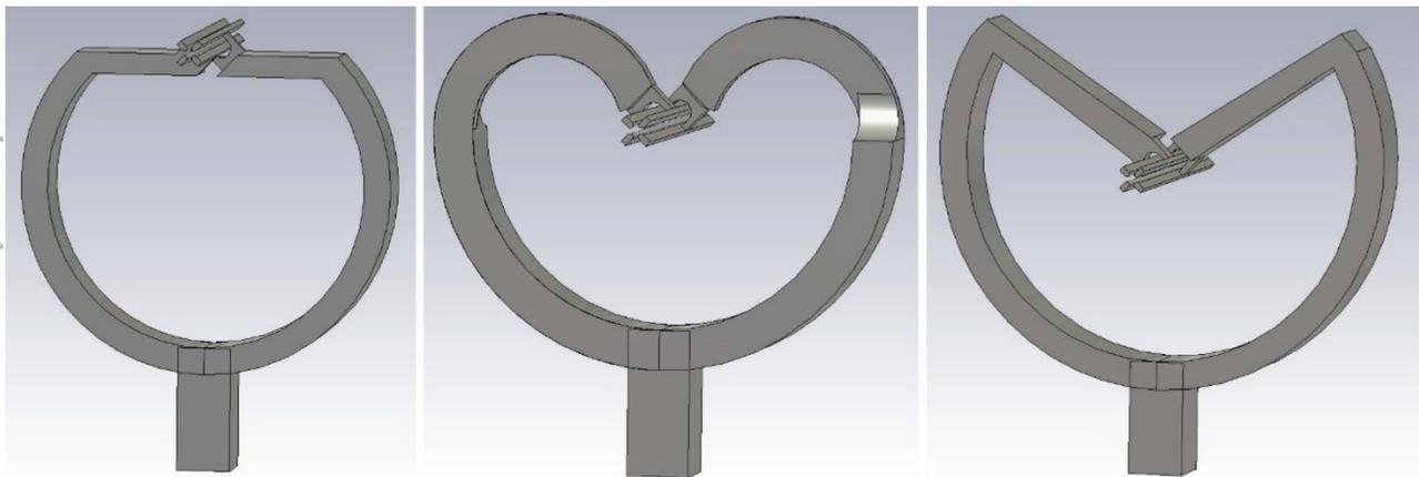
Figure 1: The three design concepts: on the left the wine glass shaped, in the middle the heart shaped and on the right the tulip shaped splitring RFQ.
