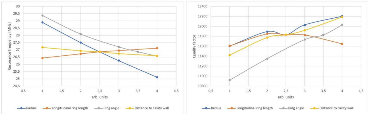
Figure 2: The influence of some geometry variations on the resonance frequency (left) and the quality factor (right) using the example of the tulip design.
