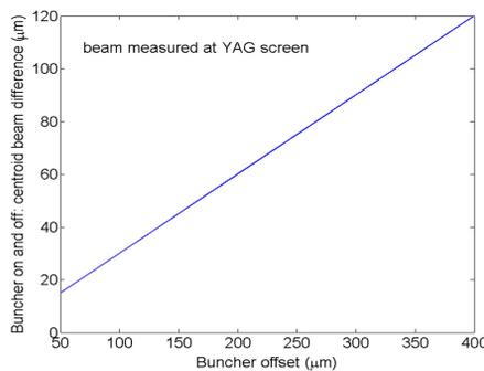
Figure 4: Transverse beam displacement difference between buncher on/off vs. buncher offset.
