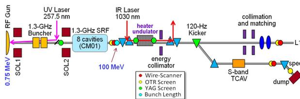
Figure 1: Schematic of the full LCLS-II injector.
