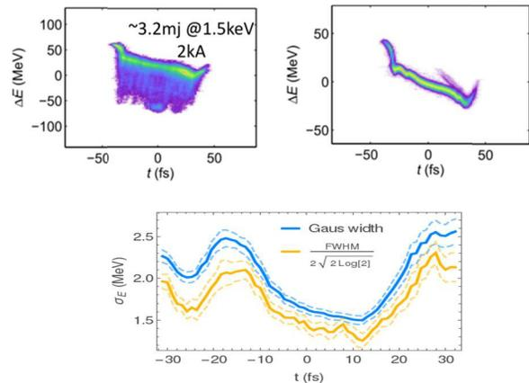
Figure 4: Measured XTCAV images with lasing (top, left), without lasing (top, right), and measured sliced energy spread along the bunch (bottom). Injector laser is from initial 2-ps pulse, then stacked to get a regular 4 ps pulse. Electron beam energy is 6 GeV.
