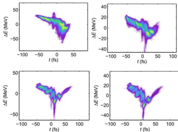
Figure 6: XTCAV images with different laser heater laser energy. Injector laser is from initial 1-ps laser, then stacked with two  $\alpha$ -BBO crystals followed by the interferometric stacker to get 8-ps pulse. Beam energy is 6 GeV.
