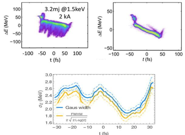
Figure 5: Measured XTCAV images with lasing (top, left), without lasing (top, right), and measured sliced energy spread along the bunch (bottom). Injector laser is from initial 1-ps laser, and then stacked with one BBO crystal followed by interferometric stacker to get 4-ps pulse. Electron beam energy is 6 GeV.
