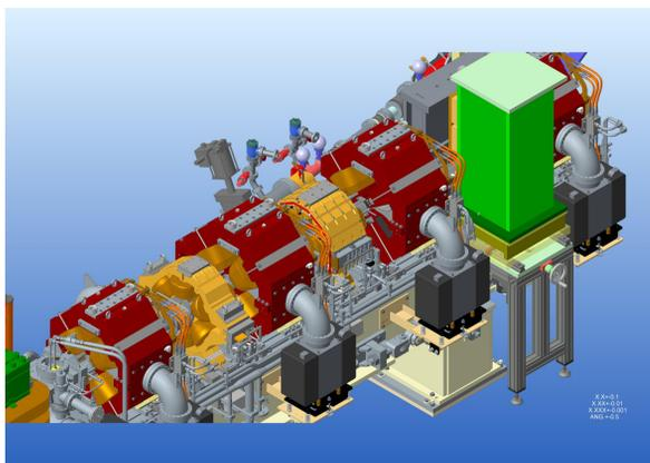
Figure 2: Model of the DIAD wiggler in place of a sextupole magnet. As there is no space available to widen the gap of the device it has been designed to be able to slide out of the electron beamline.
