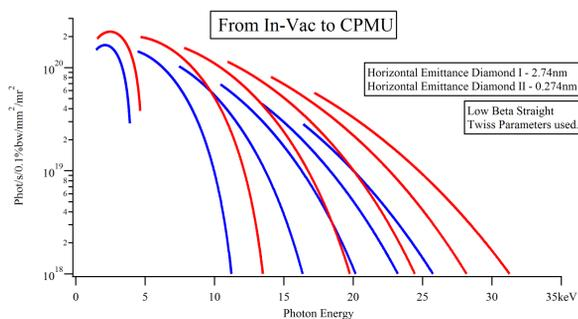
Figure 3: Brilliance plot of I03's existing structure (IVU21) and the proposed CPMU (CPMU17.6) replacement.
