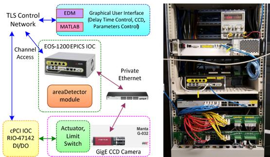
Figure 4: Block diagram and photo of upgraded BTS screen monitor system.
