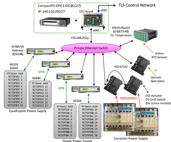
Figure 3: Architecture of new BTS control system.
