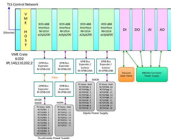
Figure 1: Architecture of original BTS control system.
