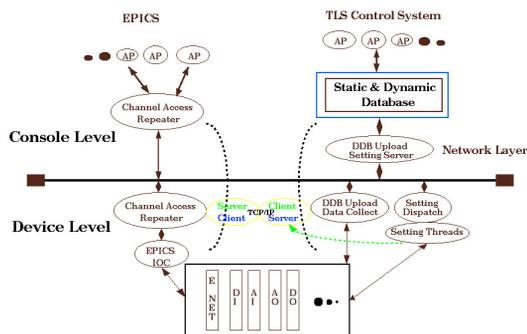
Figure 2: System architecture of EPICS IOC integrated with ILC for the TLS control system.
