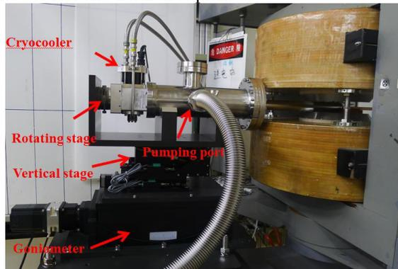
Figure 3: Hall probe calibration system
