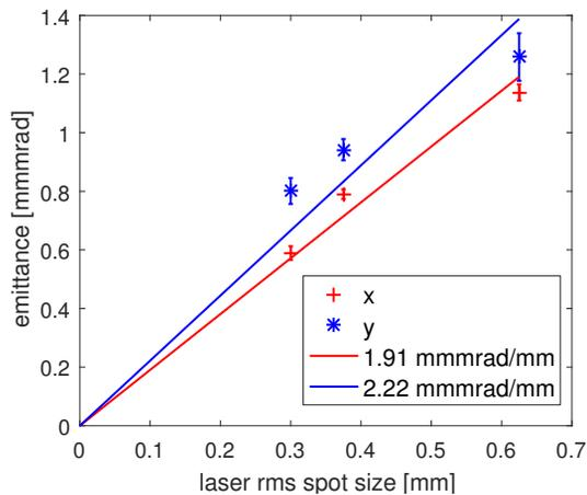
Figure 4: Emittance measurements scaling with laser spot size.
