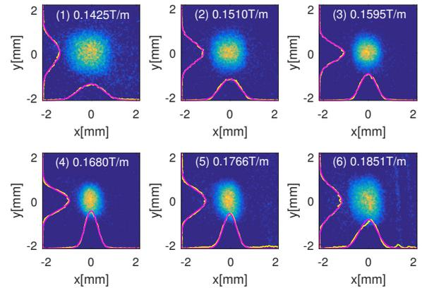
Figure 2: Six typical transverse beam images for six different quadrupole settings. The quadrupole gradients are indicated in each image. The yellow lines are the projections to the horizontal and vertical axes and the pink lines correspond to the Gaussian fits.
