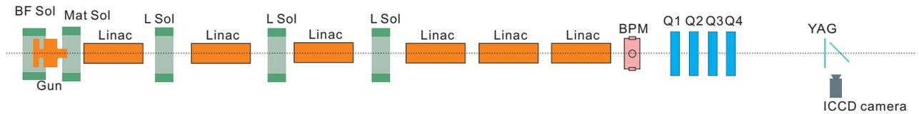
Figure 1: Schematic layout of AWA drive beamline (not to scale).
