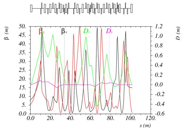
Figure 4: The Twiss function of the transport line starting from the extraction Lambertson.
