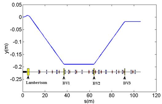
Figure 3: The layout of the two transport line in vertical plane.
