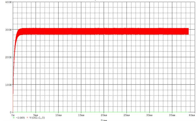
Figure 3 : PSpice result for output DC voltage.
