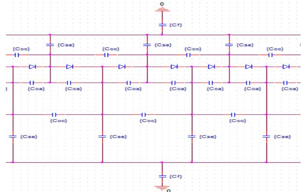
Figure 1 : simulated multiplier column circuit.
