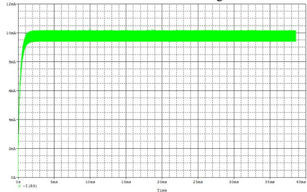
Figure 4 : PSpice result for output beam current.
