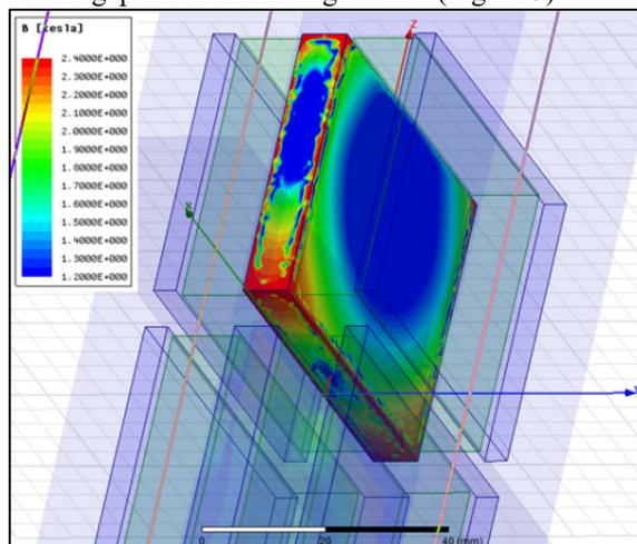
Figure 5: Model calculation of a hybrid undulator with saturation level in pole piece.
