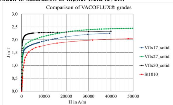
Figure 4: J-H-characteristics for various VACOFLUX<sup>®</sup>-grades.
