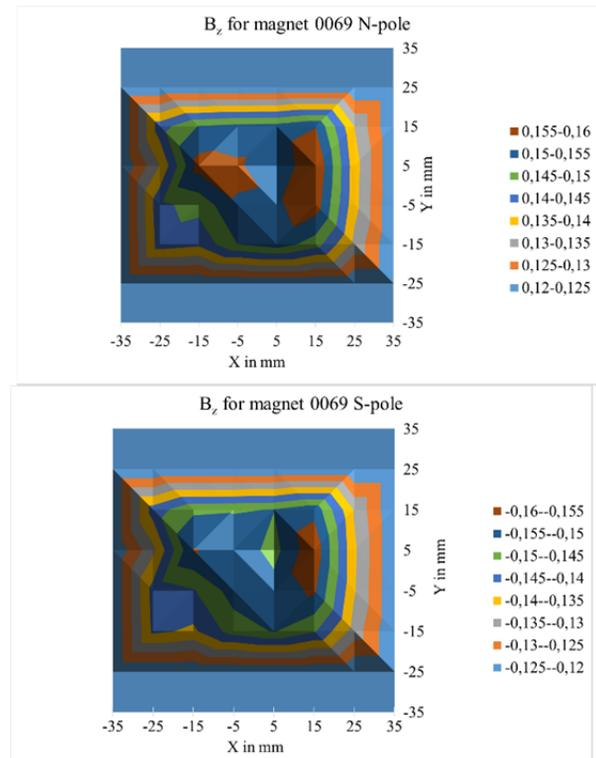
Figure 3: Field scan of  $B_z$  in T for a hybrid undulator magnet at 10 mm distance (N-pole and S-pole).
