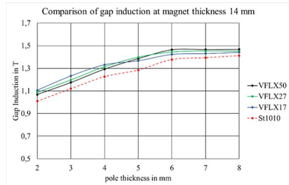
Figure 6: Comparison of gap induction for various CoFe-materials.
