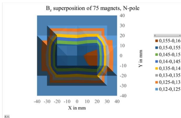
Figure 2: Simulation of the field profile for the undulator magnet recombined from measured results on 75 small pieces.
