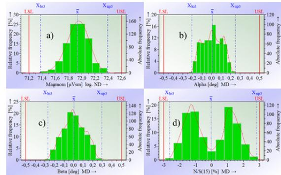
Figure 1: distribution of a) magnetic moment, angles b) Alpha, c) Beta and d) N/S-effect
