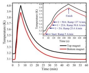
Figure 7: Temperature evolution during and after a ramp to operating current. The inset shows the temperature rise for the four ramping steps.
