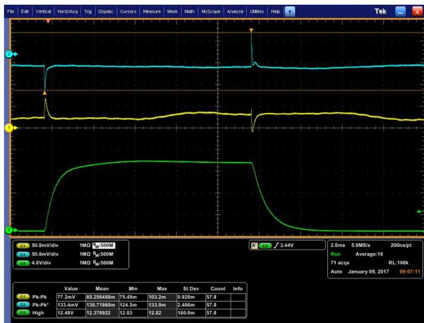
Figure 5: Beam current measurements on the LEBT line. Green: Faraday cup, yellow and blue: ACCT signals.
