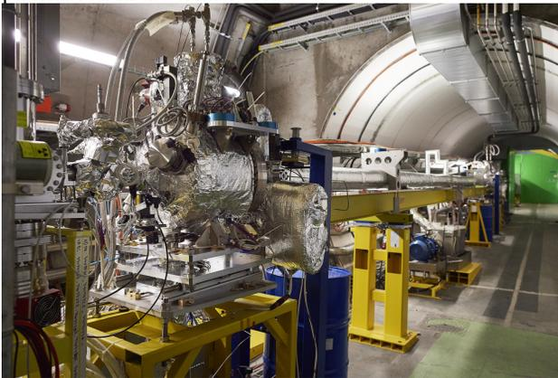
Figure 3: Looking upstream the proton beam line: Rb vapour cell with the 10 m heat exchanger and the downstream expansion chamber.
