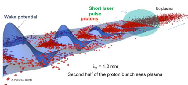
Figure 1: Simulation of the Self-Modulation Instability. The strong modulation is seen when comparing the proton distribution ahead of and behind the laser pulse.
