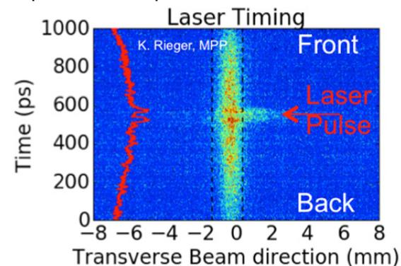
Figure 4: Measurement with the streak camera of the proton and laser beam synchronization in a 1ns window.
