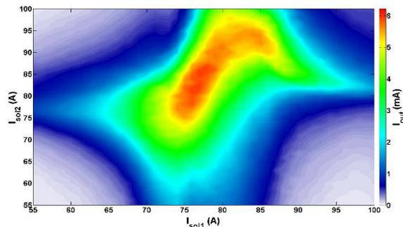
Figure 4: Transmission map with Kr injection ( $P = 2.4 \cdot 10^{-5}$  mbar, collimators aperture = 37 mm).
