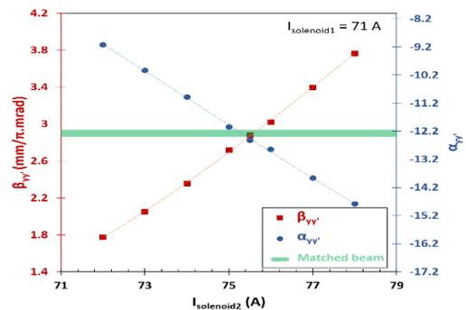
Figure 5: Twiss parameters measured at the LEBT output as a function of Solenoid 2 focusing ( $I_{\text{sol1}} = 71$  A,  $P = 2.4 \cdot 10^{-5}$  mbar, collimators aperture = 37 mm)
