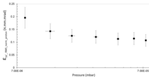
Figure 6: Measurement of the proton vertical emittance as function of the residual gas pressure after solenoid 1.
