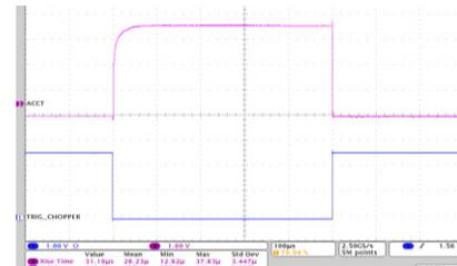
Figure 7: Macro-pulse of 500  $\mu$ s by chopping the beam at the end of the LEBT ( $P = 1.9.10^{-5}$  mbar,  $V_{\text{Chopper}} = 4$  kV).
