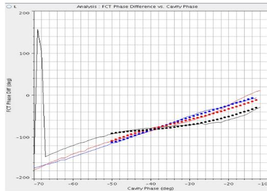
Figure 6: Plots of the DTL tank2 phase scan for nominal RF amplitude (red), 4% below nominal (blue) and 2% above nominal (black).
