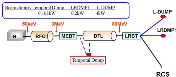
Figure 1: CSNS Linac layout.
