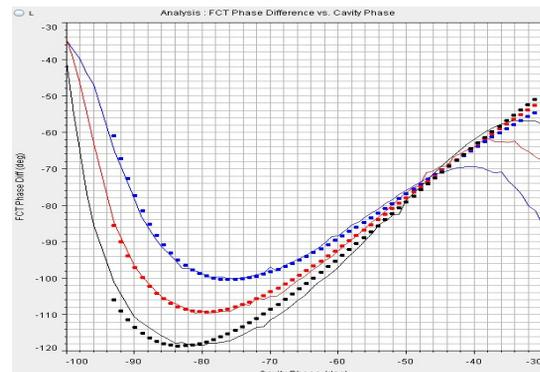
Figure 7: Plots of the DTL tank3 phase scan for nominal RF amplitude (red), 2% below nominal (blue) and 2% above nominal (black).
