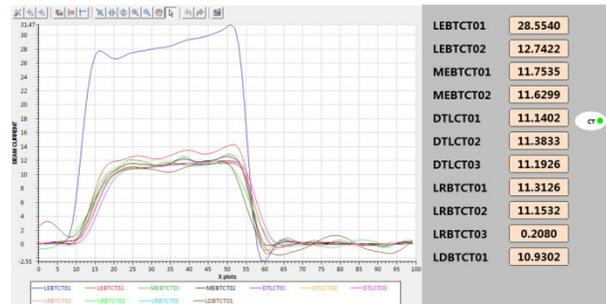
Figure 2: Current Transform signals along the Linac.
