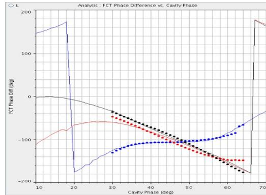
Figure 5: Plots of the DTL tank1 phase scan for nominal RF amplitude (red), 3% below nominal (blue) and 3% above nominal (black).
