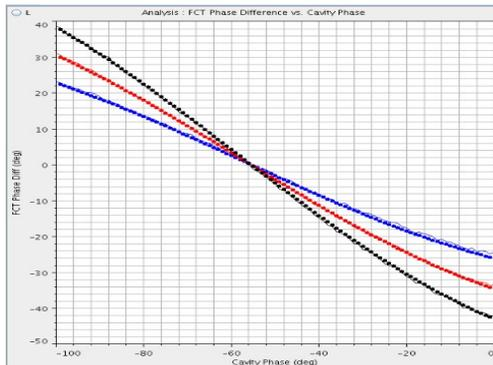
Figure 4: Measured phase differences (degrees) between two FCTs as functions of the buncher02 cavity phase.
