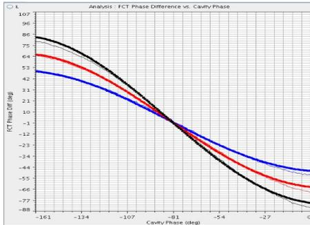
Figure 3: Measured phase differences (degrees) between two FCTs as functions of the buncher01 cavity phase.
