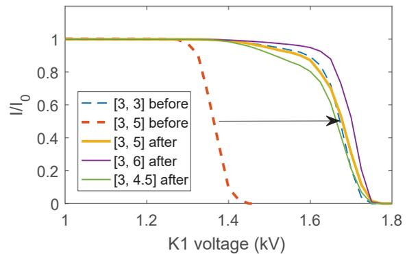
Figure 5: Comparison of dynamic aperture measurement before and after optimization for the (3, 5) case.
