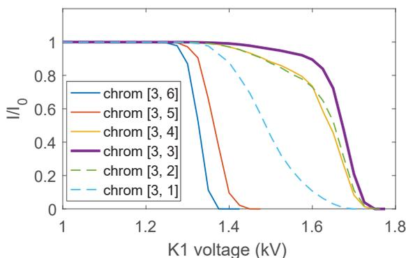
Figure 4: Dynamic aperture measurement for various vertical chromaticity values. The solution was optimized for  $C_y = 3$ . The K1 calibration is 1.212 mrad/kV.
