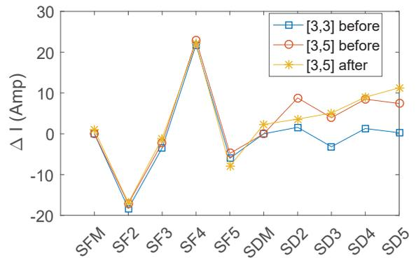
Figure 6: Sextupole changes from flat sextupole pattern before and after the optimization for the  $C_y = 5$  case.
