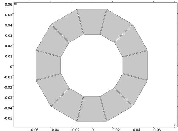
Figure 1: Geometry of the Halbach magnet used in the simulations.
