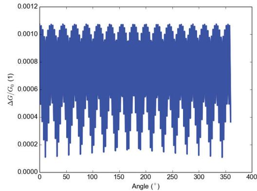
Figure 7: Gradient quality on the centre plane assuming a temperature gradient of  $1^\circ\text{C}$  as a function of angle with the horizontal axis.
