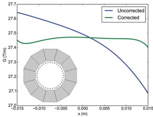
Figure 5: Gradient quality of one particular Halbach geometry; soft-iron wires are placed at the locations indicated in blue. The gradient quality is improved from 2% to 0.25%.
