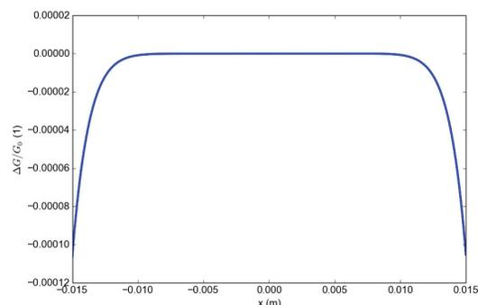
Figure 2: Gradient quality ( $\Delta G/G_0$ ) assuming a perfect geometry and magnetic properties.
