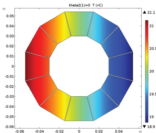
Figure 6: Temperature gradient across the magnet ( $^\circ\text{C}$ ).
