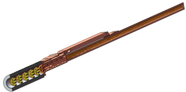
Figure 10: Rendering of the Ø3.5” KlyLac design with MBK and 2-port linac section (see Fig. 7). MBK cathode and linac focusing are not shown.
