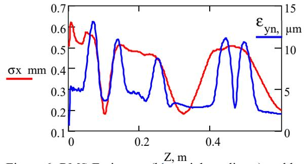
Figure 6: RMS Emittance (blue, right ordinate) and beam rms dimensions (red, left ordinate) simulated with ASTRA code for the field profile of Fig. 5 with ~7 MV/m Ez field magnitude.
