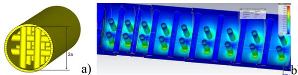
Figure 1: Cross-rod structure (a) with surface currents (b).
