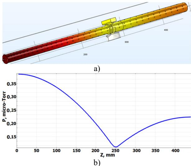
Figure 9: “Negative” volume model (a) for vacuum simulations of the cross-rod MicroLinac section of Fig. 3 having just one port for pumping. Pressure distribution simulated along the section (b).
