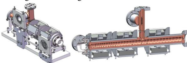
Figure 10: Finalized design of the cross-bar accelerating section.
