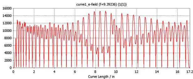
Figure 5: Absolute value of the longitudinal electric field profile plotted along the RF model of Fig. 1 for operating mode.
