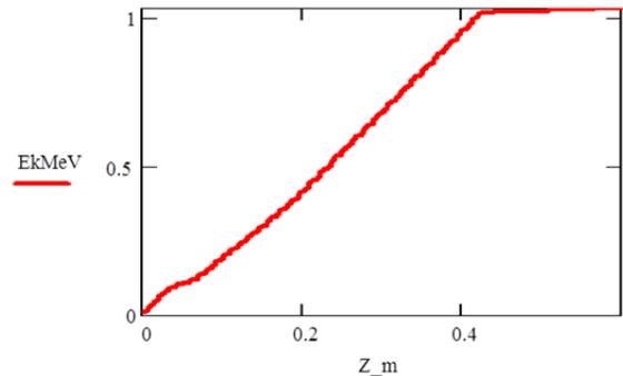
Figure 7: Beam energy gain [MeV] along the structure simulated with ASTRA code for the field profile of Fig. 5. Ez field magnitude is ~4.5 MV/m, RF power ~100 kW, capture ~15%.
