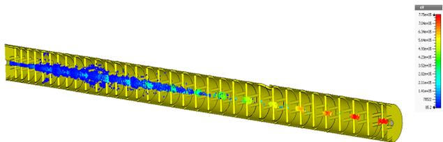
Figure 8: 3D PIC beam dynamics simulated for design of Fig. 1 with Particle Studio solver of CST Suite. Maximum on-axis longitudinal electric field is 5 MV/m, RF power is ~70 kW.
