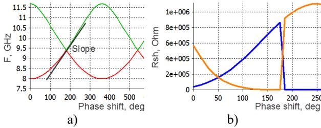
Figure 2: Brillouin diagram (a) and shunt impedance (b) vs. phase advance for a compensated cross-rod cell at 0.9c phase velocity, 3 mm aperture, and  $\varnothing$ 1.75mm rods.
