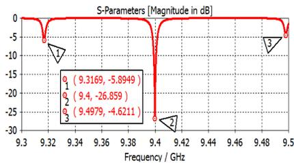
Figure 4: S11 curve simulated for the RF model Fig. 1.
