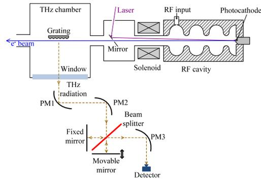
Figure 1: Schematic experimental set-up showing: photocathode gun, 3.6-cell RF cavity, grating, sapphire window and the Michelson interferometer.
