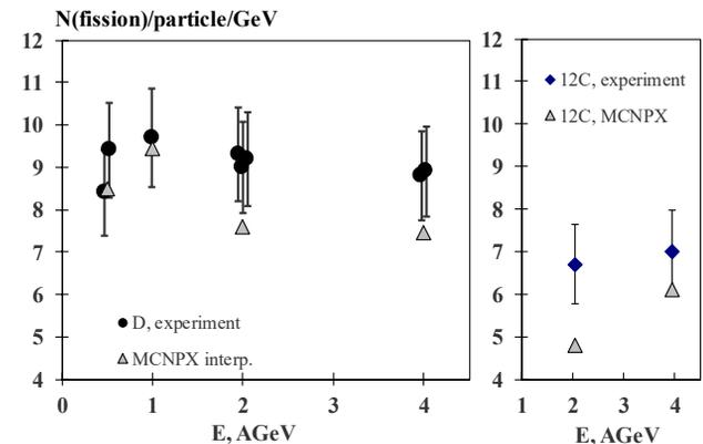
Figure 3: Integral numbers of  $^{\text{nat}}\text{U}(n, f)$  reactions in the volume of uranium target as a function of beam energy.
