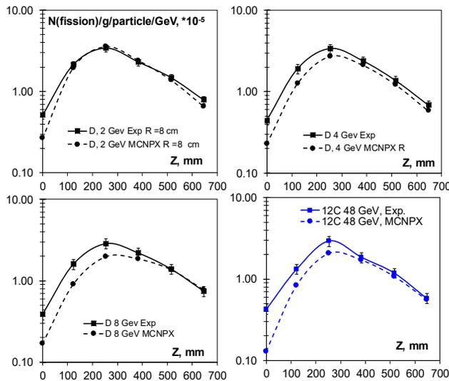
Figure 5: Experimental and Monte Carlo calculation Axial distributions of  $^{\text{nat}}\text{U}$  fission rates for samples at radial distances of  $R = 8$  cm.
