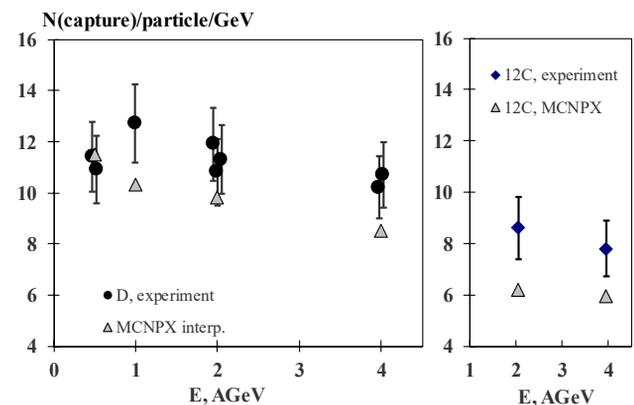
Figure 4: Integral numbers of  $^{238}\text{U}(n, \gamma)$  reactions in the volume of uranium target as a function of beam energy.
