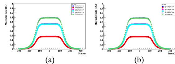
Figure 5a-5b: The magnetic field measurement results at -27.5mm and +27mm on the x axis of the magnet for the results both TUBITAK National Metrology Institute and Scanditronix. These results are consistent within error bars.
