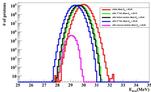
Figure 4: The beam kinetic energy change along the METU-DBL generated by a TURTLE simulation using an initial 30MeV with 1% dispersion. The final proton beam kinetic energy is still within the standard.
