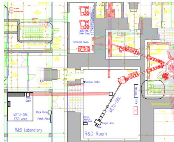
Figure 1: Drawing of R&D room, technical room and R&D laboratory at the PAF. METU-DBL is in the R&D room while the chiller group is shown in the technical room and the control of the METU-DBL will be done from the ESD area in the R&D laboratory.
