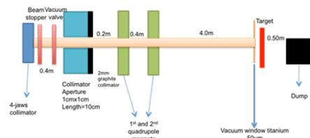
Figure 6: The schematic of the preliminary test setup of the METU-DBL. A collimator is necessary to protect the magnets.
