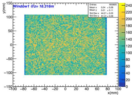
Figure 3: The beam size at the target position generated by a TURTLE simulation. Required beam size is satisfied.
