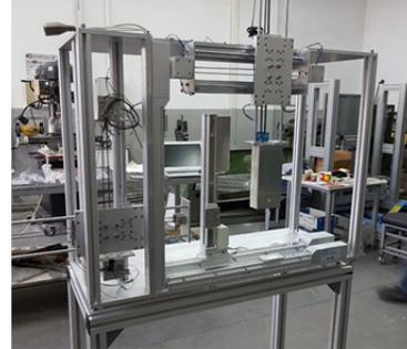
Figure 9: The table for the detectors and the mounting for the device under test. The detectors must scan the beam area in order to check the uniformity of the beam distributions.
