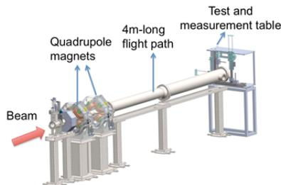
Figure 7: The technical drawing of the preliminary test setup with the test and measurement table at the target position.
