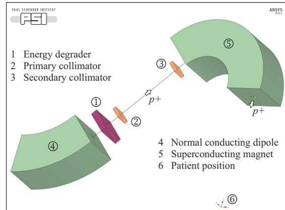
Figure 1: Beamline layout of “degrader on gantry” concept.
