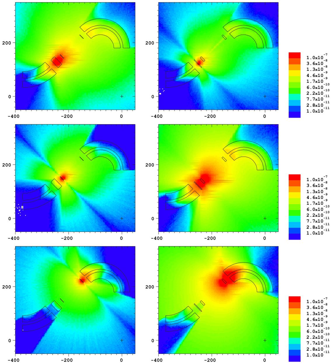
Figure 4: Neutron dose [ $\mu\text{Sv}$ ] per primary proton for the case of the beam impinging onto the degrader (1<sup>st</sup> row), primary (2<sup>nd</sup> row) and secondary collimator (3<sup>rd</sup> row) when degrading to 70 MeV (left column) and to 230 MeV (right column).
