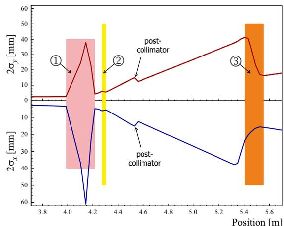
Figure 2: The beam envelope of  $2\sigma_{x,y}$  simulated for the energy setting of 70 MeV for the EDS layout of the COMET cyclotron. Same labels as in Fig. 1. The losses at the post-collimator, downstream from the primary collimator, were included into the losses at the primary collimator.
