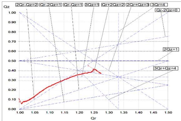
Figure 3: Tune diagram.
