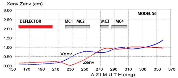
Figure 10: RMS envelopes of the extracted beam.
