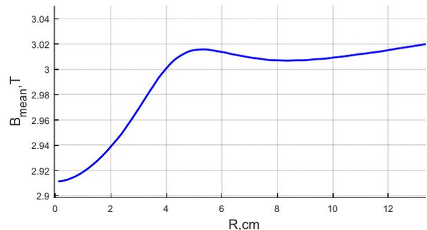
Figure 6: Average magnetic field in the center.
