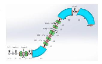
Figure 7: Layout of the gantry beamline with downstream scanning (Scanning magnets and nozzle not shown).
