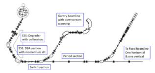
Figure 1: Layout of the beamline.
