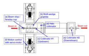
Figure 3: Schematic view of the multi-wedge degrader.
