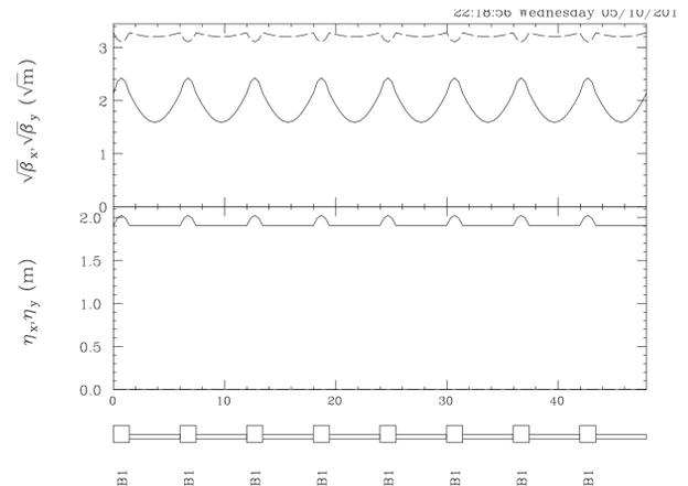
Figure 3: The lattice functions of the 400 MeV ring. Since the spiral angle is zero and no reverse bends are installed, vertical focusing force is generated by only edge focusing of the main magnets.
