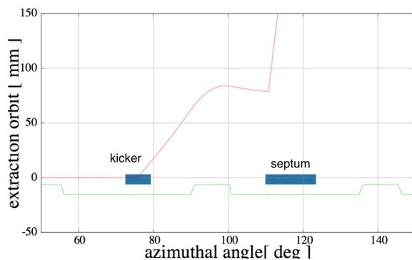
Figure 6: A scheme of the beam extraction from the 400 MeV ring. The kicker magnet kicks the beam by 30 mrad with the magnetic field of 2 kG to make 75 mm turn separation at the septum magnet. The phase advance between the kicker and septum magnet is about 90°. Both of them should be moved by remote controlled mechanism inside the vacuum chamber in order to extract the beams at different energies.
