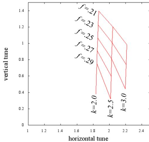
Figure 2: The tune variation with respect to the field index  $k$  and the packing factor  $f$ . Red lines are contour of those parameters. To avoid integer resonances and keep the beam excursion small, we have chosen parameters  $k$  and  $f$  as 3.0 and 0.23, respectively.
