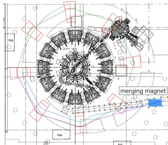
Figure 7: Footprint of the extracted beams. Red lines show the main magnets of the 400 MeV ring. The blue and purple lines show the trajectories of protons extracted at 200 MeV and 400 MeV, respectively. These lines are crossing at the merging magnet indicated by a blue box. By adjusting the magnetic field of the merging magnet, the beams with any energies between 200 and 400 MeV can be extracted and transported through the same beam line to the KUCA.
