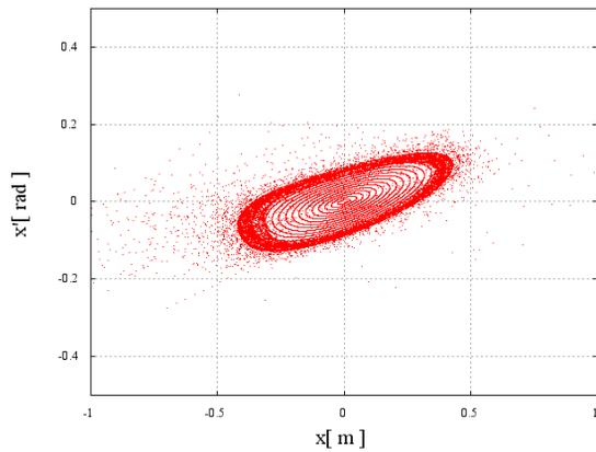
Figure 5: The horizontal phase space structure. Particle tracking has been performed through 10 000 turns using 4th order Runge-Kutta solver. A large stable region is guaranteed compared with the beam size estimated as a few cm.
