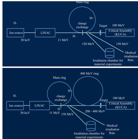
Figure 1: The schematic diagram of the FFAG Accelerator Complex. The upper is the current configuration and the lower is one of the future plans adopting a newly designed 400 MeV ring.
