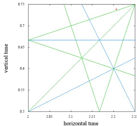
Figure 4: The tune diagram of the 400 MeV ring. Blue and green lines are 3rd and 4th order resonance lines, respectively. The red cross is the operating point. Since it is close to the resonance excited by skew octupoles, it may be changed according to further investigations.
