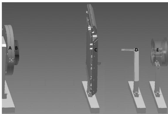
Figure 2: Scheme of the geometrical setup and positioning of the beam measuring instruments of the delivered beam in air: A= FCT, B= IIC, C= Multistrip Ionization Chamber, D= synthetic single crystal diamond, E= Faraday Cup.
