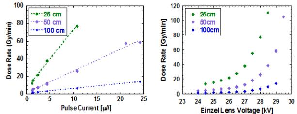
Figure 7: Proton dose rate vs the pulse current ( $\mu\text{A}$ ), left, and vs the einzel lens voltage (kV), right, measured by the synthetic single crystal diamond.
