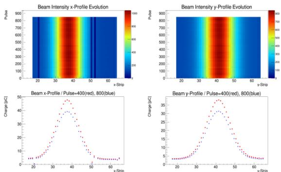
Figure 6: Beam Intensity x and y profiles versus all pulses (upper plots) and for two predefined pulses (lower plots).
