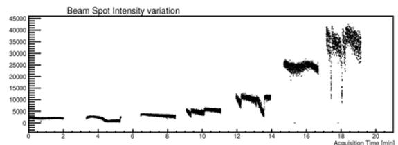
Figure 4: Total charge recorded on the chamber, for each beam pulse (single point in plot) while the beam intensity is changed on purpose. The unit on the y axis is arbitrary.
