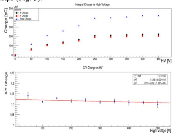
Figure 3: Top: total charge collected by the x and y strips as a function of the chamber bias current. Bottom: x and y axis charge ratio; the red line represent a linear fit. The about 10% greater collected charge along x is related to the slightly larger size of the x strips respect to the y ones.
