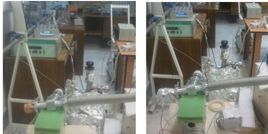
Figure 6: Coupling cell after brazing (a) Vacuum level during bake out, (b) bake out setup.
