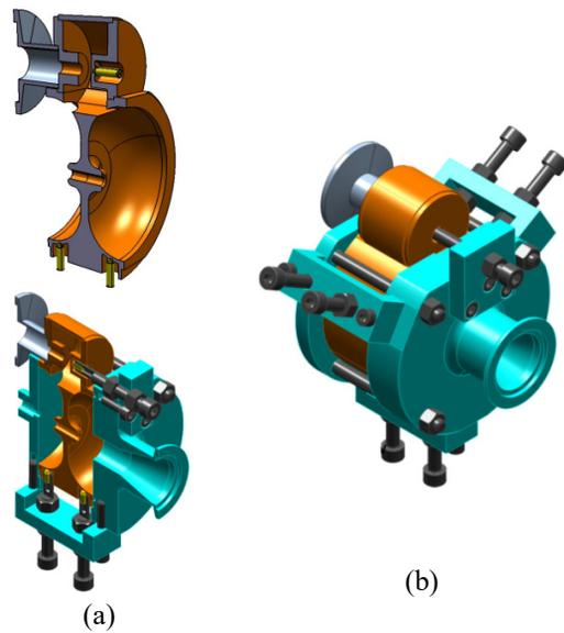
Figure 4: schematics of cavity with tuning mechanism (a) Cut view (b) Full view.
