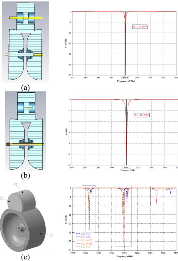
Figure 3: Simulation of expected results of measurement and tuning (a) tuning of accelerating half cells (b) tuning of coupling cell (c) frequency spectrum after tuning with different Antenna penetration Length (best on 1.5 mm).
