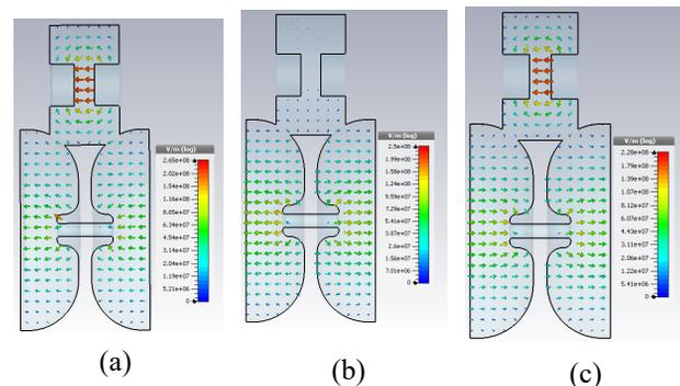
Figure 1: Electric field profiles of 0,  $\pi/2$ ,  $\pi$  modes.
