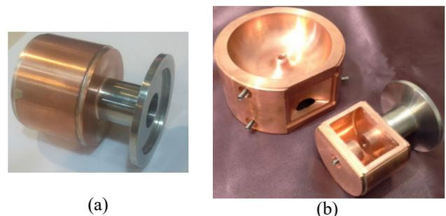
Figure 5: (a) Brazed coupling cell (b) whole of parts for final brazing.
