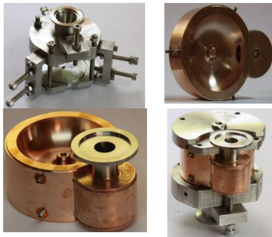
Figure 7: Side coupled brazed prototype.
