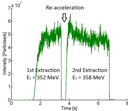
Figure 4: Carbon spill on two different energy-levels in the HEBT-line. Measured with ionisation chamber immediately after the synchrotron. First part of spill:  $E_1 = 352$  MeV/u. Second part of spill:  $E_2 = 358$  MeV/u. Re-acceleration takes place between the two parts of the spill.
