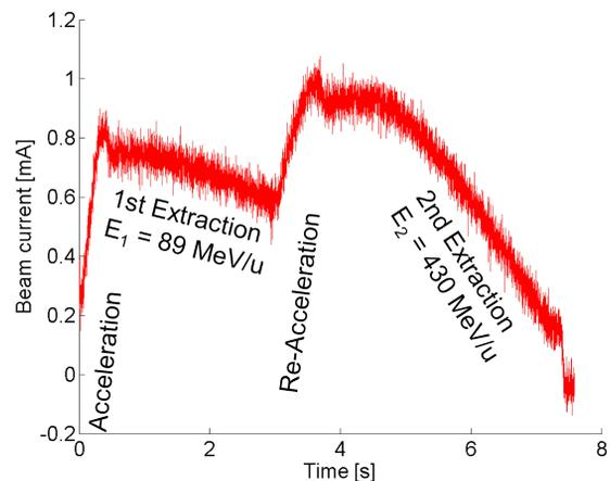
Figure 3: Beam current in the synchrotron measured by a DCCT for a carbon spill in the new multi energy operation mode. First acceleration to:  $E_1 = 89$  MeV/u. Second energy level:  $E_2 = 430$  MeV/u. The beam current rises in the first standard acceleration phase as well as during re-acceleration and decreases in the phases for slow extraction.
