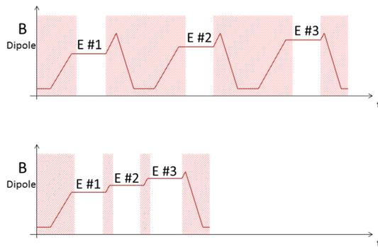
Figure 2: Synchrotron dipole current in old and new synchrotron operation mode, schematically. Phases without beam availability at the treatment room are shown in red. Top: In the present irradiation scheme each synchrotron cycle can provide one extraction energy ( $E\#1, 2, 3\dots$ ) only. Bottom: The goal of the new and currently investigated *Multi Energy Operation Mode* is to irradiate several consecutive iso energy slices with very short interruptions.
