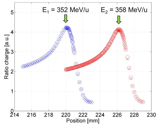
Figure 5: Depth dose curves (*Bragg-Peaks*) measured with ionisation chambers in a water column for two different energy levels. X-Axis: Range in mm. Y-Axis: Peak-plateau ratio of ionisation. Red: Carbon beam at 358 MeV/u. Blue: Carbon beam at 352 MeV/u. Crosses: Reference measurement for single energy operation scheme. Dots: Measurement for multi energy operation mode, both energies available within one synchrotron cycle. The resulting Bragg-peaks are identical for both scenarios.
