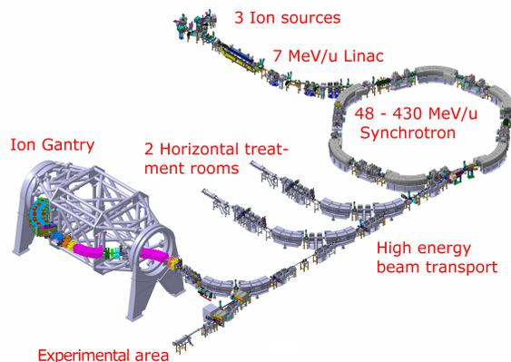
Figure 1: HIT accelerator complex. The synchrotron based accelerator can deliver 4 different types of ions to 3 treatment rooms and one experimental room in therapy quality.
