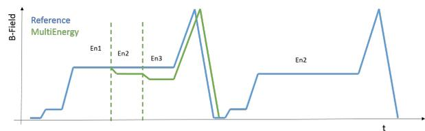
Figure 3: Magnetic cycle in the synchrotron. Blue: reference as implemented; Green: example of Multi energy spills.
