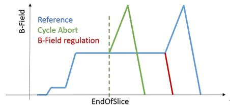
Figure 1: Magnetic cycle in the synchrotron. Blue: reference as implemented; Red: with magnetic field regulation; Green: example of Cycle Abort for a slice requiring delivering of roughly 30% of the particle accelerated in a cycle.
