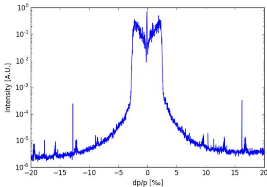
Figure 4: Beam  $\frac{dp}{p}$  after the phase jump used to prepare the beam for extraction [14], as derived from measurement of the  $\Sigma$  spectrum of the horizontal Schottky monitor.
