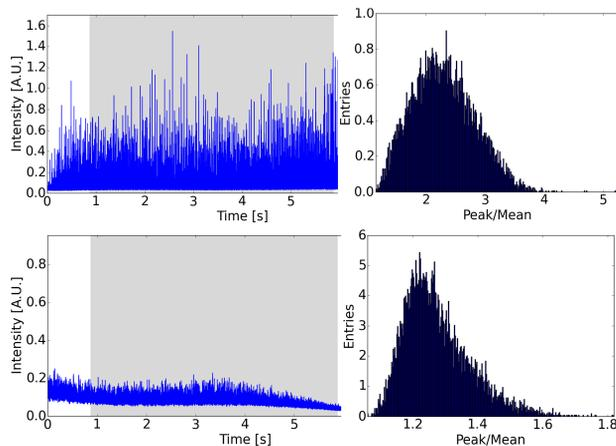
Figure 2: Left: spill structure of the extracted beam at 252MeV; right: peak to average intensity distribution. Top: reference; bottom: with RF-Channeling, empty bucket at 4kV and +10kHz offset respect to the revolution frequency.
