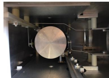
Figure 6: NMR cartridge is running on the rails between the kicker plates. Input jumper is visible at the top.
