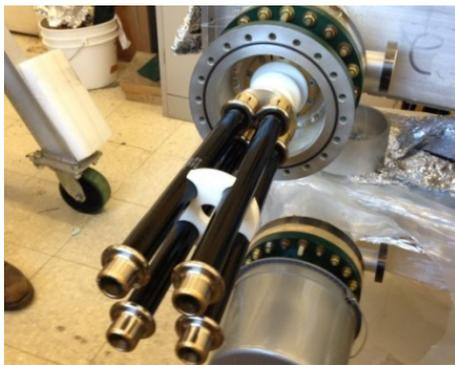
Figure 3: The Kicker input. Four load resistors are Kanthal tubular resistors, 50Ω each. Cylindrical protective cover removed. Inner volume is filled with Fluorinert FC-40.
