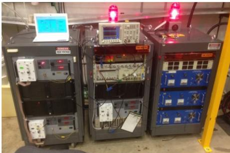
Figure 7: Charging pulser tower (left), the control tower (center) and the thyatrons PS tower (right).
