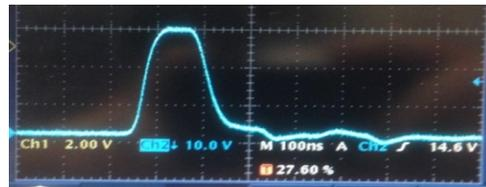
Figure 9: The current measured at the kicker input at Fermilab.  $4 \text{ kA}@\text{max}$ , 100ns/div.
