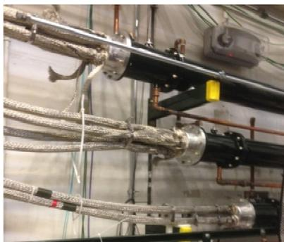
Figure 8: Output side of Blumlein generators.
