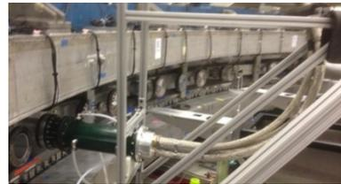
Figure 10: The input into the g-2 ring chamber, kicker #3.
