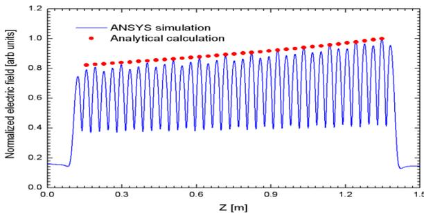
Figure 2: The electric field amplitude distribution along the accelerating structure.
