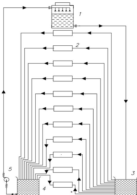
Figure 7: Layout of the 40 C thermostabilization system.
