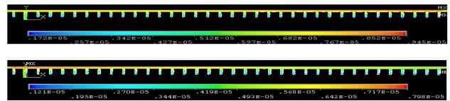
Figure 5: Transversal deformations along the structure without (upper) and with (lower) beam.
