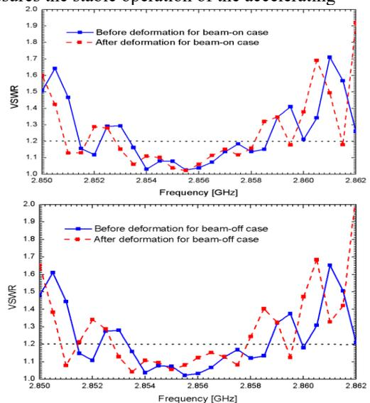
Figure 6: VSWRs of the structure versus frequency for both beam-off and beam-on cases.
