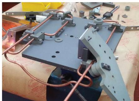
Figure 4: Tooling for shaping of the liner cooling tubes.
