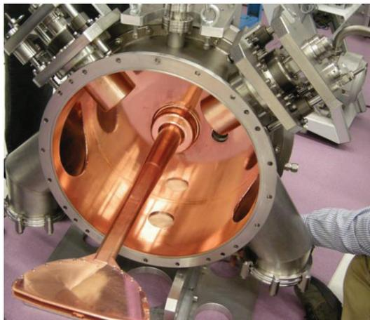
Figure 2: Stem and dee mounted on the resonator.
