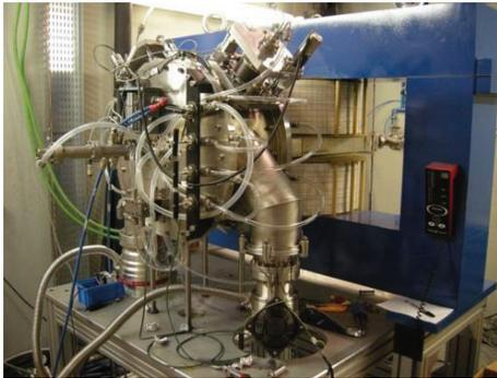
Figure 5: Cavity and magnet at the RF laboratory bunker.
