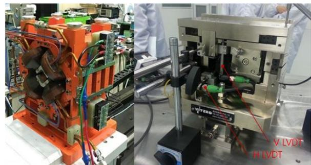
Figure 4: Q6 Magnet and quad mover.
