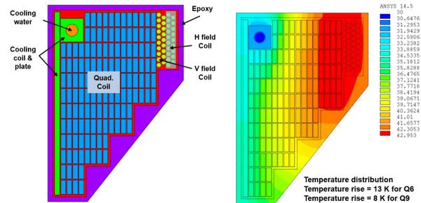
Figure 3: The conductor cross section and temperature distribution of quadrupole magnet Q6 and Q9.
