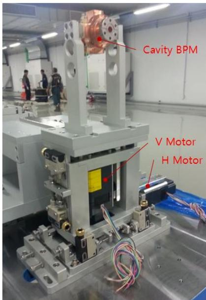
Figure 2: 3D view of cavity BPM Mover.
